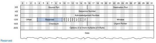
Has no use in previous TCP versions. Must be set to 0 so that future TCP versions can use the field if needed.
