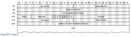
• Used to terminate a TCP connection without proper teardown.
