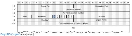
If the flag is set, the data in the current TCP segment is immediately forwarded to higher layers starting with the first byte up to where the urgent pointer field points.
