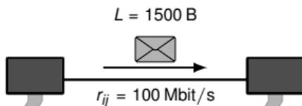
$$t_s = \frac{L}{r} = \frac{1500 \cdot 8 \text{ bit}}{100 \cdot 10^6 \text{ bit/s}} = 120 \mu\text{s}$$
