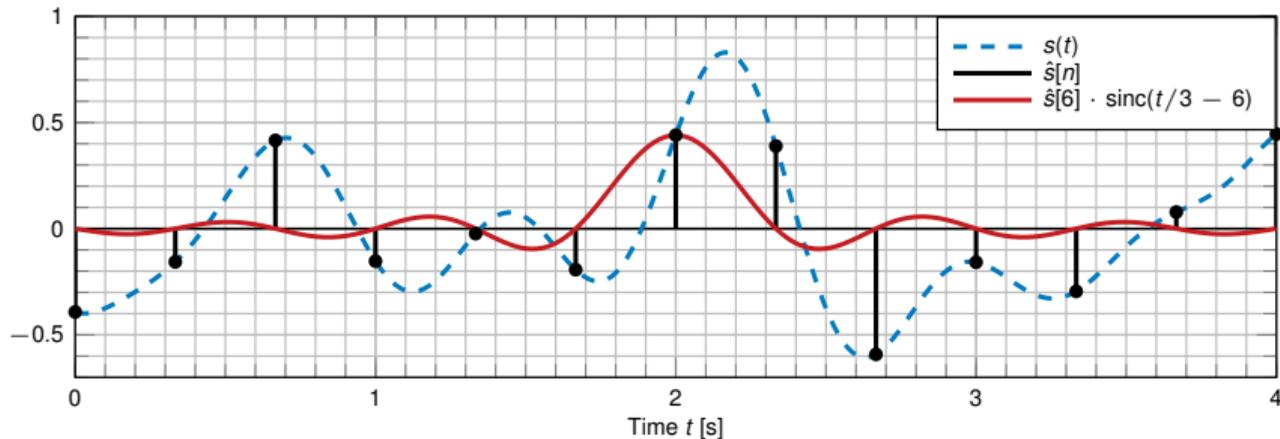
Figure 3: Each sample  $\hat{s}[n]$  serves as a weight for the reconstruction function.
