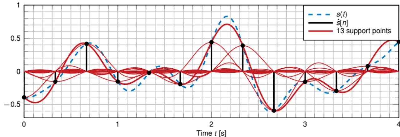
Figure 3: The sum of the weighted functions approaches the original signal depending on the number of summing elements.
