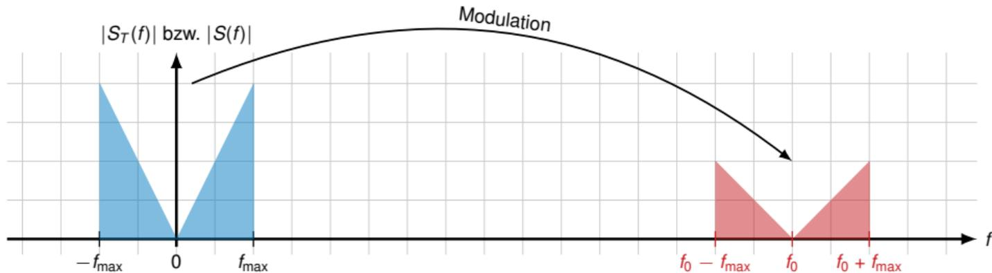
Spectrum of the transmit signal  $s_T(t)$  in the basebandSpectrum of the bandpass signal after modulation  $s(t)$
