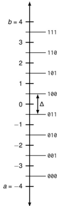
**Example:** Linear quantization within the interval  $I = [-0.5; 0.5]$  mit  $N = 3$  bit:
