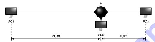
Figure 2.1: Waternet consisting of three computers and one distribution unit.
